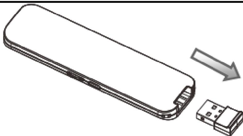
(Plug the USB receiver into the computer's USB port.)
